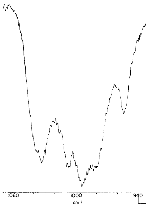
Figure 3. Infrared spectrum in the V=O region of V_2O_2Cl_4(Hmhp)_3 as a 1% KBr pellet.
